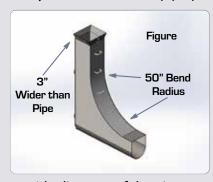
radius of 50". This minimum radius will provide a smooth transition during the installation process.
