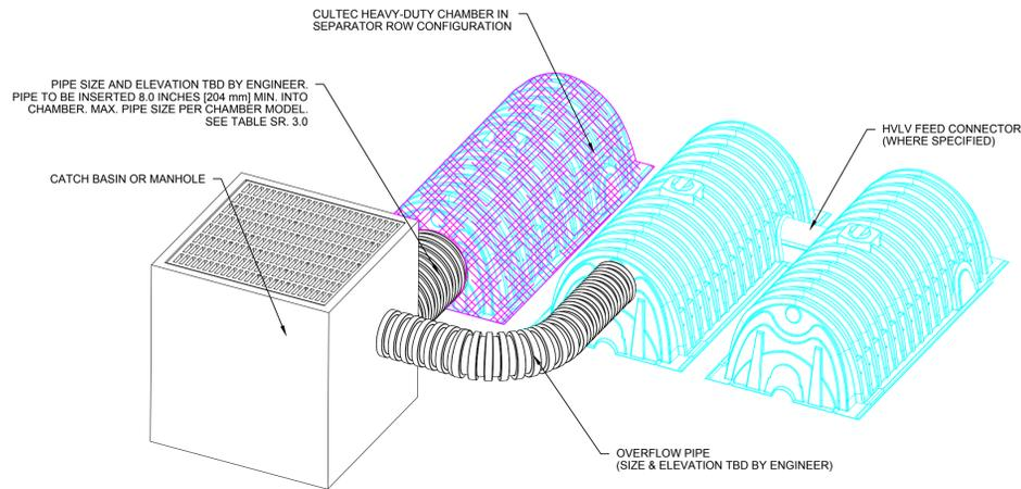
**TYPICAL SEPARATOR ROW CONFIGURATION INLET CONNECTION**
