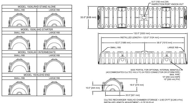
CULTEC RECHARGER 150XLHD CHAMBER STORAGE = 2.65 CF/FT [0.245 m<sup>3</sup>/m] INSTALLED LENGTH ADJUSTMENT = 0.75 [0.2 m] ALL RECHARGER 150XLHD HEAVY-DUTY UNITS ARE MARKED WITH A COLORED STRIPE FORMED INTO THE PART ALONG THE LENGTH OF THE CHAMBER. SIDE PORTAL ACCEPTS CULTEC HYLV FC-24 FEED CONNECTOR.
