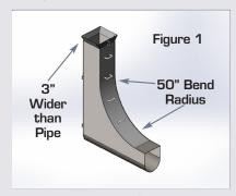
radius of 50". This minimum radius will provide a smooth transition during the installation process.
